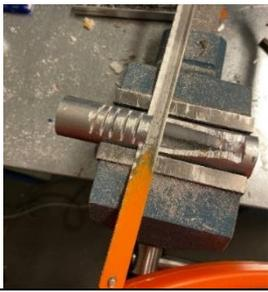
A close-up view of a hand saw cutting through a metal rod held in a vise.                                                |
