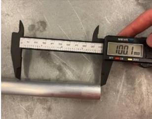
A digital caliper is used to measure the diameter of a metal rod. The display shows 10.0 mm.                               |
